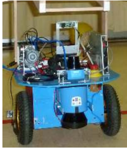
Fig. 2. The robot equipped with Sick LMS100 and TiM300 laser scanners, Logitech C270 camera, and the motorized fork lift.
