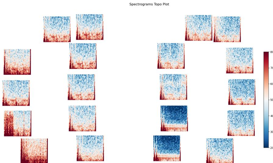
**Figure 19. Alpha response for each electrode of the Enten headphones.** Participants had their eyes open and closed for 30 seconds each. This procedure was repeated twice
