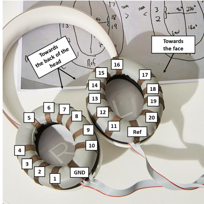
**Figure 1. Enten headphones prototype.** There are 10 electrodes on both ear pads, plus the reference (Ref) and the ground (GND) electrodes. The electrodes are dry, active, and made of a conductive mesh that wraps around the ear pads.
