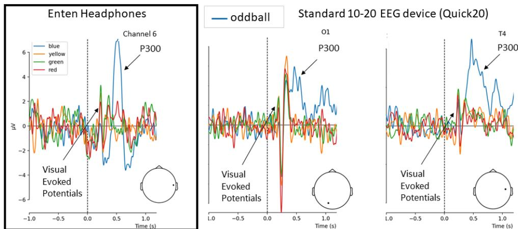
**Figure 5. Evoked response from Oddball experiment for Quick20 and Enten.** The participant was placed in front of a computer screen with different color words appearing on the screen and was instructed to press a key every time the word “BLUE” appeared on the screen, and to ignore all other words. This experiment was performed twice, once on the Quick20, and once on Enten.
