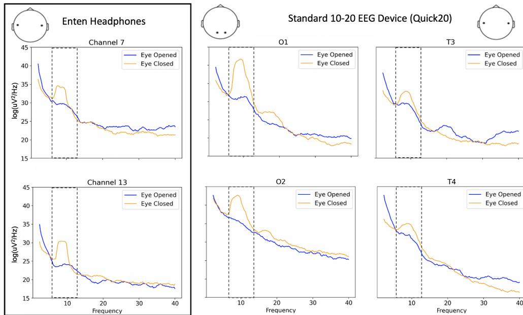
**Figure 3. Power spectral density (PSD) for the eyes opened and closed experiment.** PSD is calculated based on 4 seconds windows from the recorded data of Enten headphones (left) and Quick20 (middle and right) of the same subject. The PSD of the eyes-closed state is shown in orange, while the PSD of the eyes-opened state is shown in blue.
