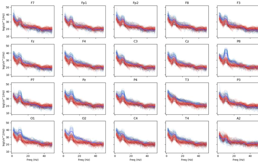
**Figure 20. Headset comparison by channel.** Eyes closed alpha for Enten Channel 17 (red) versus a commercially available 10-20 system (Cognionics Quick20, blue). Same subject in both cases. PSDs are calculated based on 100 seconds of eyes closed data. Translucent lines indicate individual epochs (2 second duration, 50% overlapping), and solid lines denote the average across these epochs.
