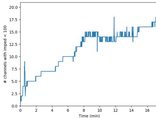
**Figure 21. Number of channels with low impedance (<100 kΩ) at as a function of time.** Electrodes require several minutes to settle. This informed us to require subjects to wear the headphones for a few minutes before starting the experiment.
