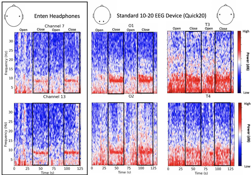
**Figure 2. Spectrogram from the eyes opened and closed experiment.** This recording is from a single participant during 2 minutes of experiment, where the eyes are open for 30 seconds followed by 30 seconds of eyes-closed state. The procedure is repeated twice, as recorded in Enten headphones (left) and Quick20 (middle and right panels correspond to the occipital and temporal channels, respectively).
